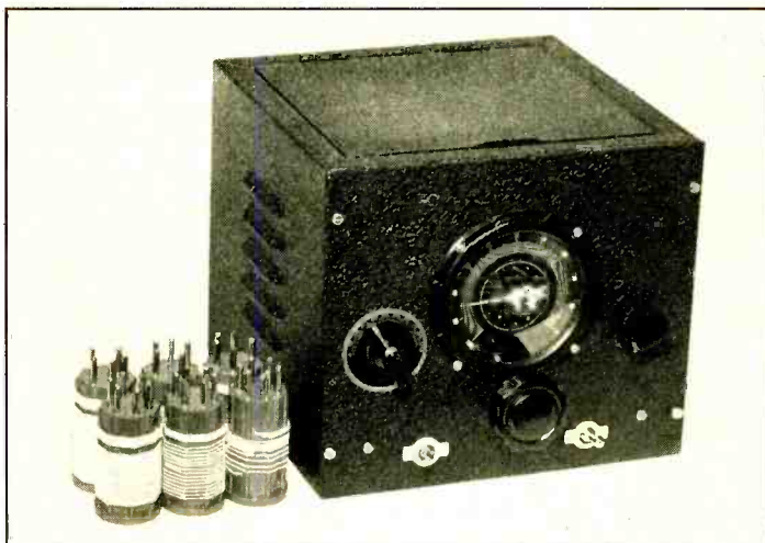
Figure 1. Front view of the converter installed in its metal cabinet. The coils for the 80-, 40-, and 20-meter bands are shown to the left of the unit. The front panel controls are: oscillator bandset, bandspread, and detector tuning; the left-hand switch is for filament voltage and the one to the right controls the b.f.o.
